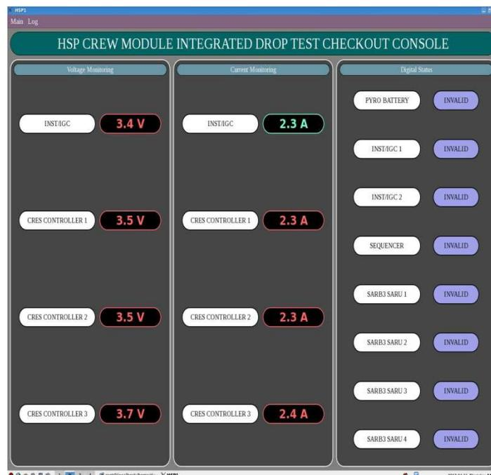
Fig.3.GUI at PC side displaying data from DAQ.
