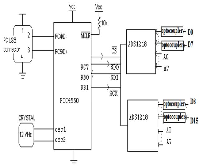
Fig. 1. Hardware block diagram.
