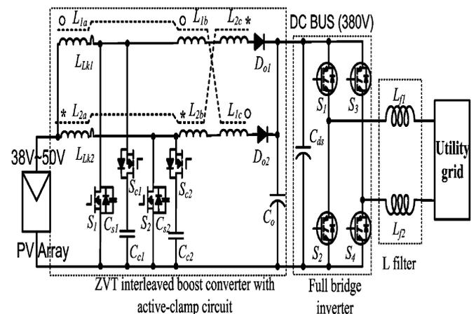
Fig. 4. Proposed grid-connected PV power system.
