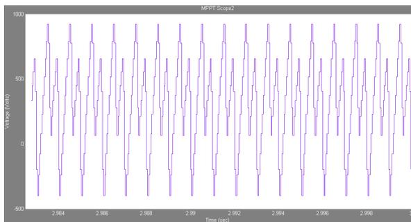
Figure 14. Output of the Solar Unit (or) MPPT Voltage.
