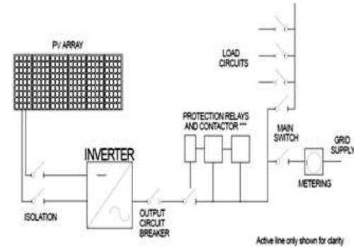
Fig.3. A grid connected system with basic main components of the system.
