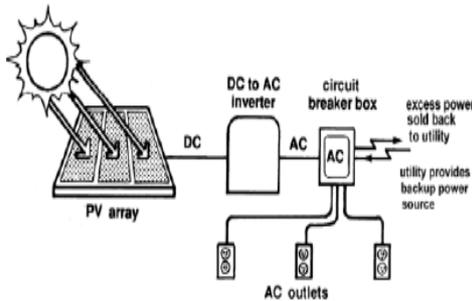
Fig.1. Grid Connected PV systems.
