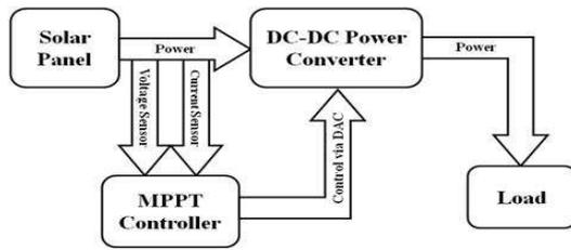
Figure 8. DC – DC converter for operation at the MPPT.
