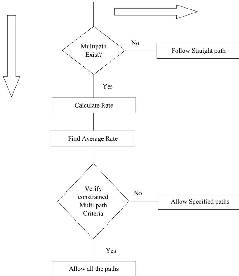
Fig.1 Multipath Flow Diagram
